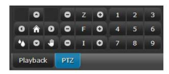
When a camera has PTZ capabilities the PTZ tab will be clickable. Clicking on this tab will bring up the interface to the left.
